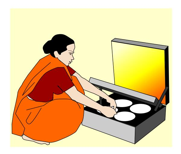
out of locally available materials. They were often small cardboard devices suitable for cooking a single meal when the sun was shining, or wood and glass boxes built into the sunny side of a house with thermal time constants of a number of hours. Thus they could cook even when the sun was behind a cloud.
