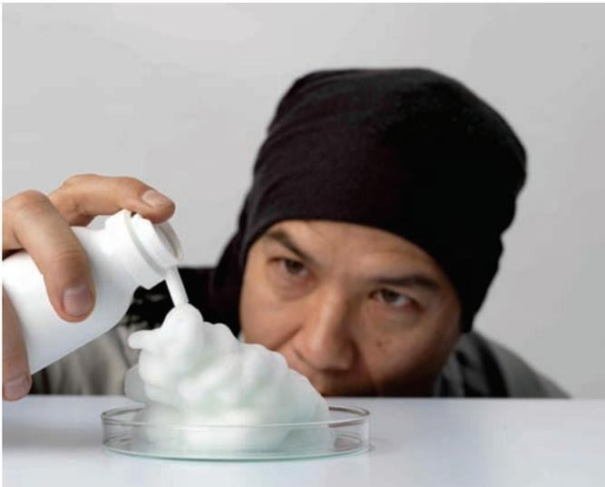
VOCs are organic chemical compounds - propane and/or butane. It is under pressure remain in liquefied state inside an aerosol can along with a foaming agent. The mixture is expelled as a vapour through the nozzle when the valve is opened. The expanding gas puffs the foaming agent up to froth.
